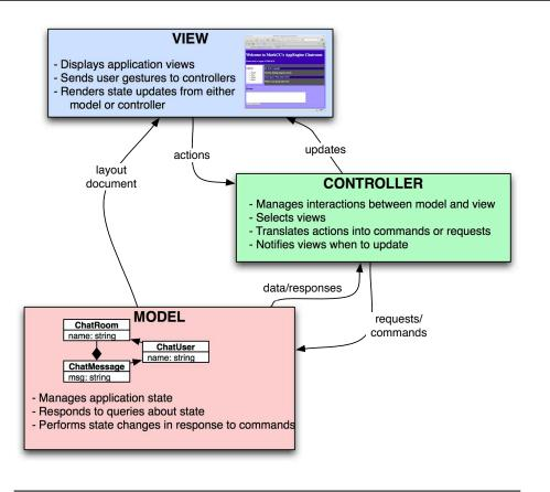
Figure 8.1: The structure of a cloud MVC application
